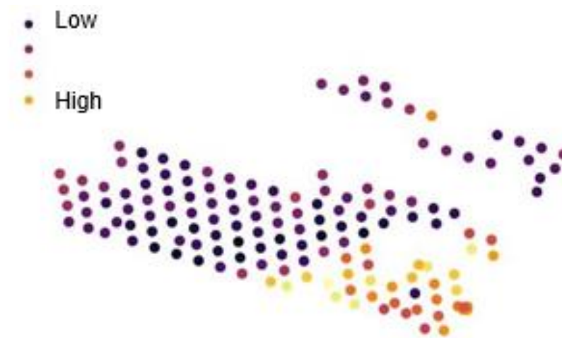
Figure 7. Horizontal variation in rock UCS value. Plotting a colour-coded map of the third quartile UCS value for each blasthole helps visualize the lateral distribution of rock hardness across a drilling pattern. This example corresponds to the pattern shown in 3D in Figure 6. Dark colours indicate low UCS rock, corresponding to the location of the fault. Lighter colours to the south of the fault indicate harder rock.
