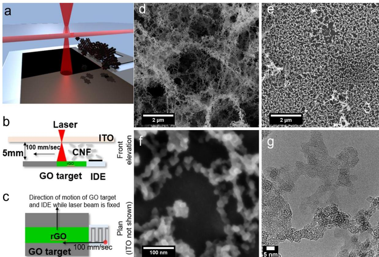
**Fig1** a) Fabrication setup in 3D, b) side and c) top view of processing steps of the fabrication. SEM image of d) carbon aerogel diffusion barrier, e) active layer after removal of diffusion barrier, f) high magnification image of active layer, showing individual carbon clusters, g) HRTEM of LDCA diffusion barrier layer.
