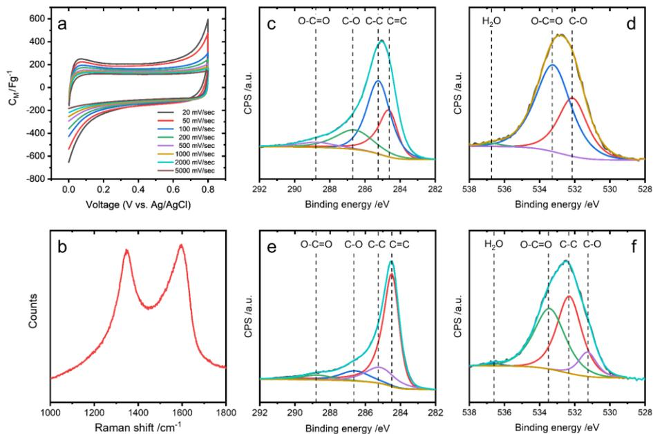
**Fig2** a) Cyclic voltammographs at different cycling rates of active LDCA layer, b) Raman of annealed active LDCA layer c) Deconvoluted XPS spectra of C1-peak of diffusion barrier layer, d) Deconvoluted XPS spectra of O-peak of diffusion barrier layer, e) Deconvoluted XPS spectra of C1-peak of active LDCA layer f) Deconvoluted XPS spectra of O-peak of active LDCA layer.
