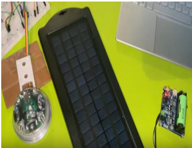
Fig. 7: Connection of solar panel to waveshare solar power management board
