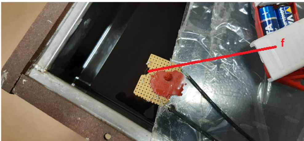
Figure 12. Photograph of the PD corona spark source (f).
