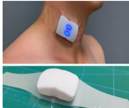
Figure 2: The wireless Doppler ultrasound patch
