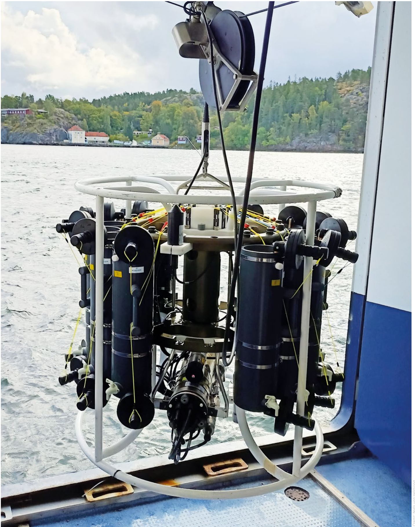
Figure 5.2 A Conductivity-Temperature-Depth (CTD) device. The combination of CTDs with dissolved oxygen sensors and Niskin bottle collections facilitates the continuous measurement of oxygen in the water column.
