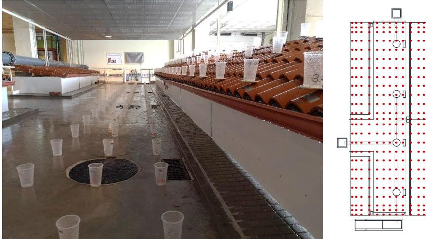
Figure 3. Grid of 325 vessels was located over the whole facility to accurately measure rainfall intensity and its spatial uniformity.
