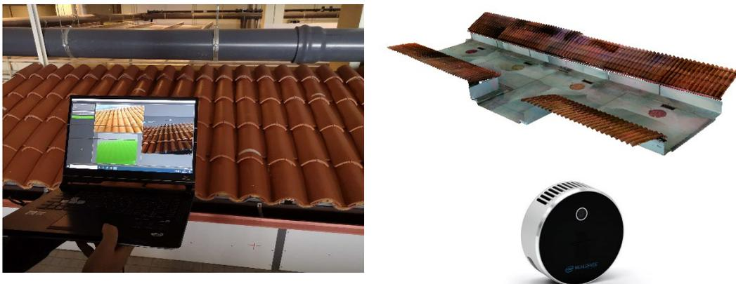
Figure 4. 3D LiDAR reconstruction of roofs and surface (left) using the Intel® RealSense™ LiDAR Camera L515 sensor (right down) and 3D model obtained (right up).
