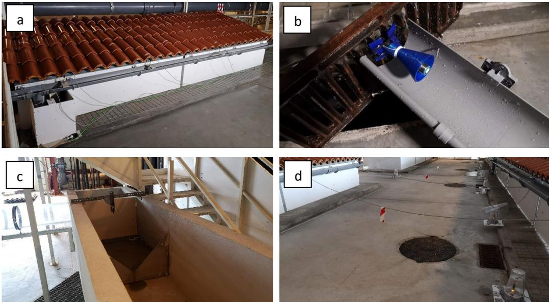
Figure 5. Experimental set-up to measure roof discharges (a), inlet discharges (b), outfall flow (c) and surface depths (d).
