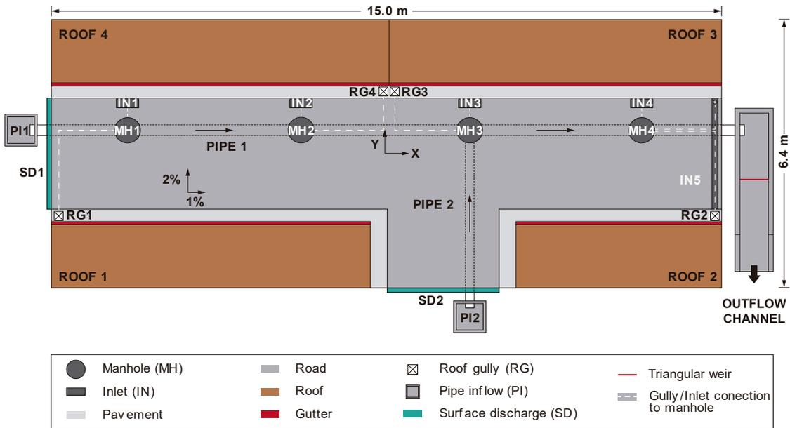
Figure 2. Scheme of the urban drainage facility
