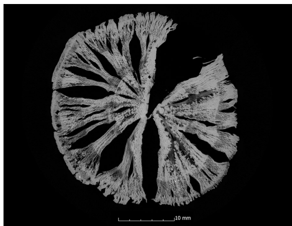
Fig. 10 \mu CT cross section of the alder sample treated with lactitol/trehalose (A11-LaTr) with cell collapse in the wood structure
