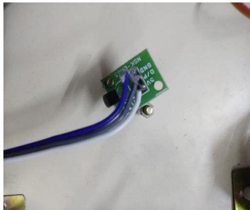
Figure.2. Temperature sensor (LM35)
