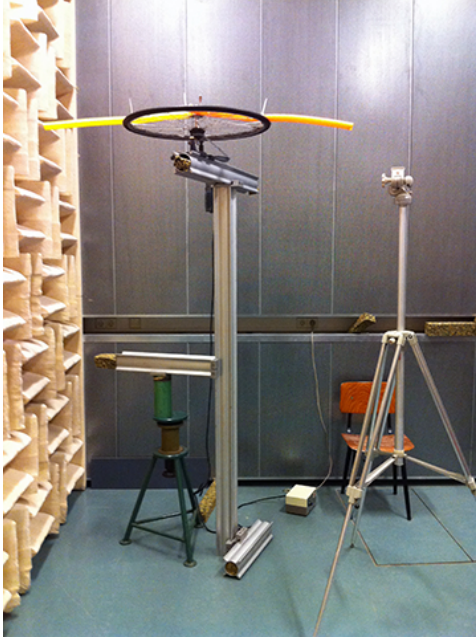
Figure 3. Overview of the set-up with reflecting floor.
