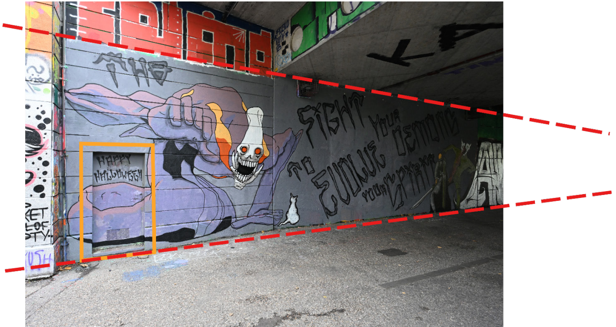
Figure 5. Photograph taken around Halloween in November 2021. The photograph exhibits typical distortions occurring in conventional photos. The perspective distortion is highlighted with two converging dashed red lines. The orange rectangle shows an example of topographic displacement caused by a door in the wall. The lens distortion is made visible with the red dashed line. While the wall bottom is a straight line in the real world, its image is slightly curved.
