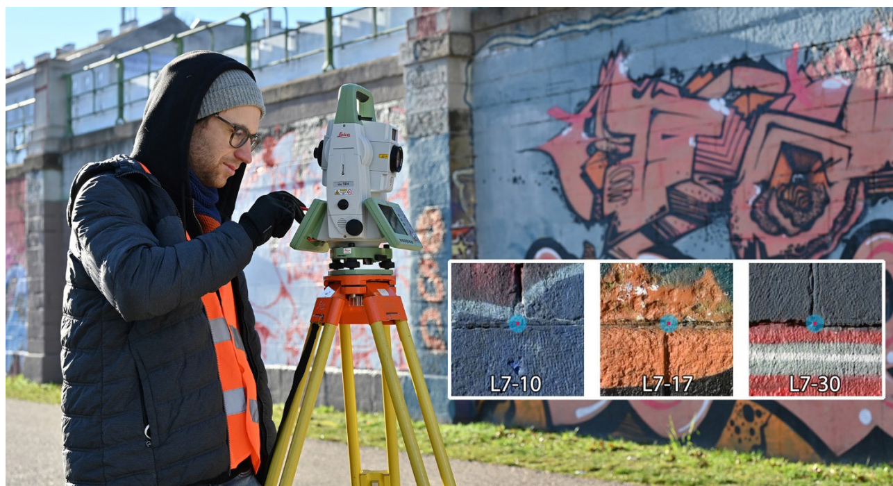
Figure 8. Operating the Leica Viva TS16 total station. The inset on the lower right displays three typical GPs.
