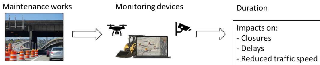
Figure 5 Process flow for collection of PIs for duration of inspection and maintenance works
