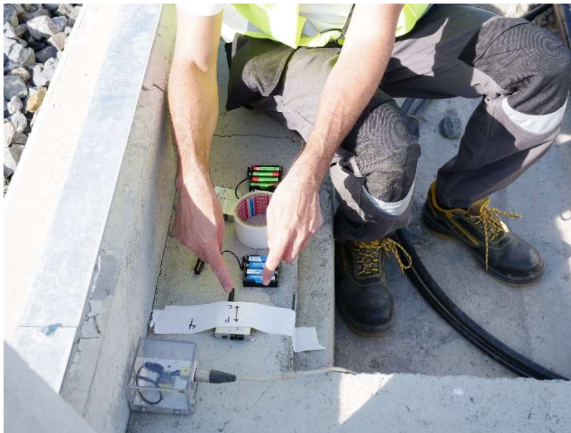
Figure 64. Preparation of accelerometers during testing
