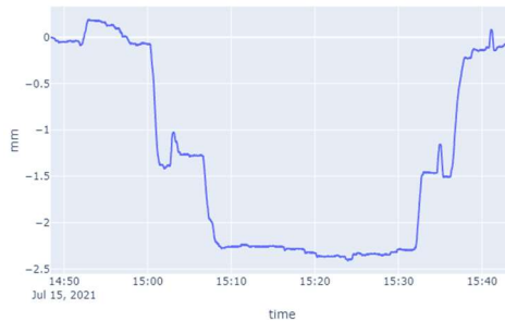
Figure 55. Vertical displacements at the midspan 3 (static load test)
