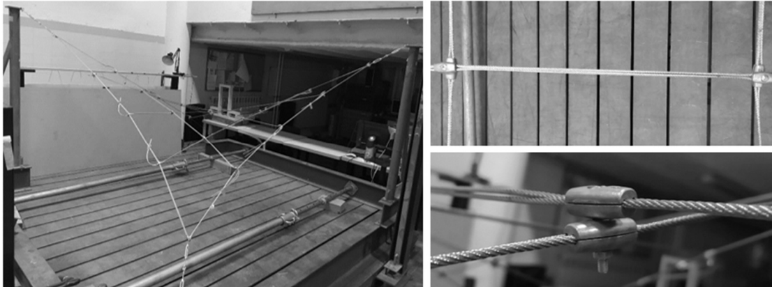
Figure 35. Prestressed cable net
