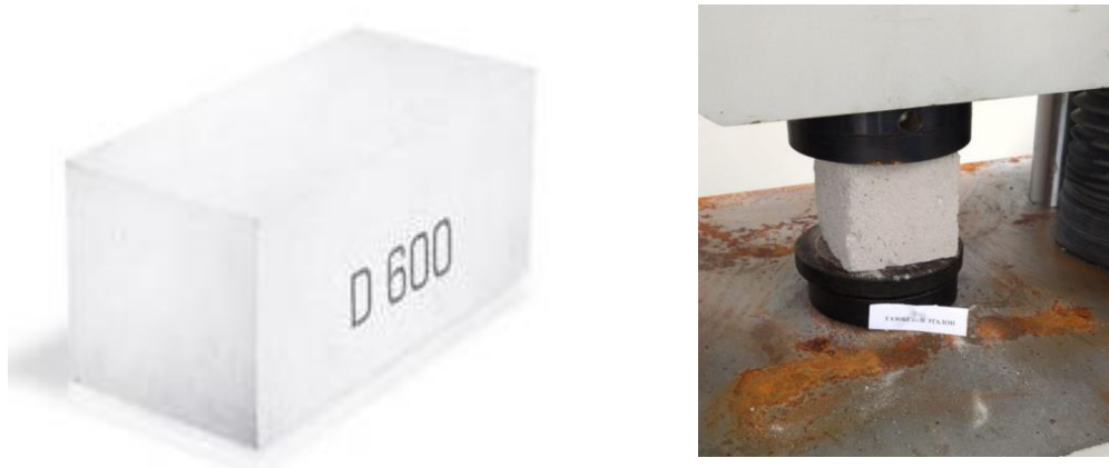
2-picture. Strength parameters of lightweight concrete with a volume of 600 kg/m 3 .
