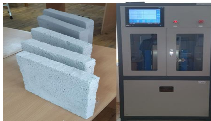
3-picture. Samples of 300*300*50 mm for determining thermal-physical parameters of lightweight concrete.
