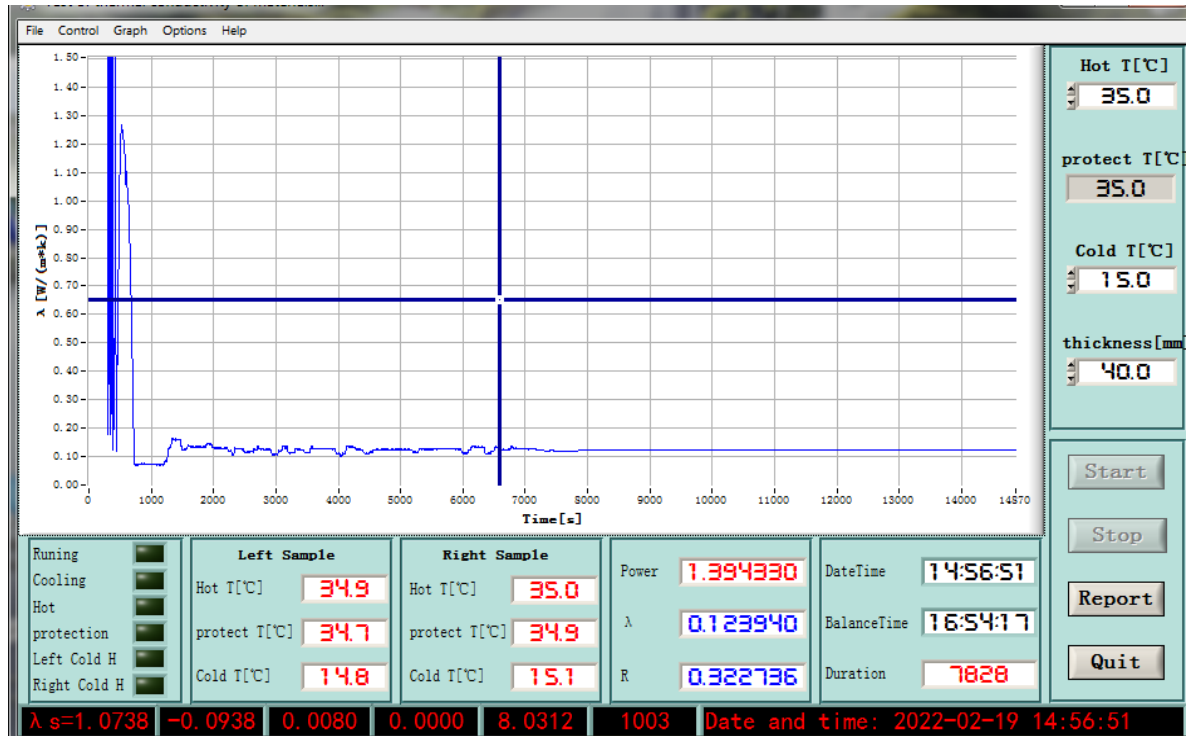
picture. Thermal and physical parameters of lightweight concrete with a volume mass of 600 kg/m 3 .
