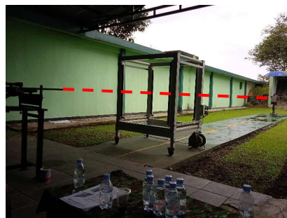
Fig. 7. Ballistic experiment schematic: a – distance illustration; b – real experiment set up environment; c – multilayered armor system mounted on the mannequin
