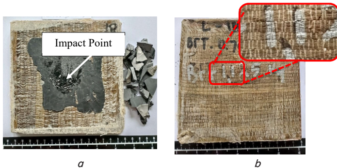
Fig. 14. Macrostructure of 6SiC+10R: a – front side; b – rear side
