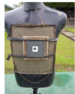
Fig. 7. Ballistic experiment schematic: a – distance illustration; b – real experiment set up environment; c – multilayered armor system mounted on the mannequin
