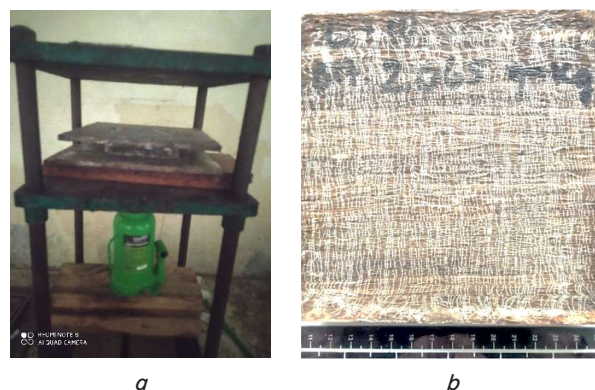
Fig. 5. Composite molding process: a – hydraulic; b – ramie composite (150×150 mm in dimensions)
