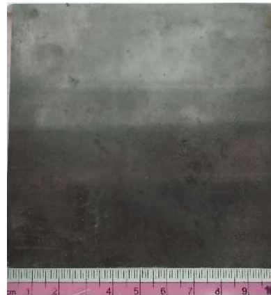
Fig. 4. Silicon Carbide (SiC) material (100×100 mm in dimensions)
