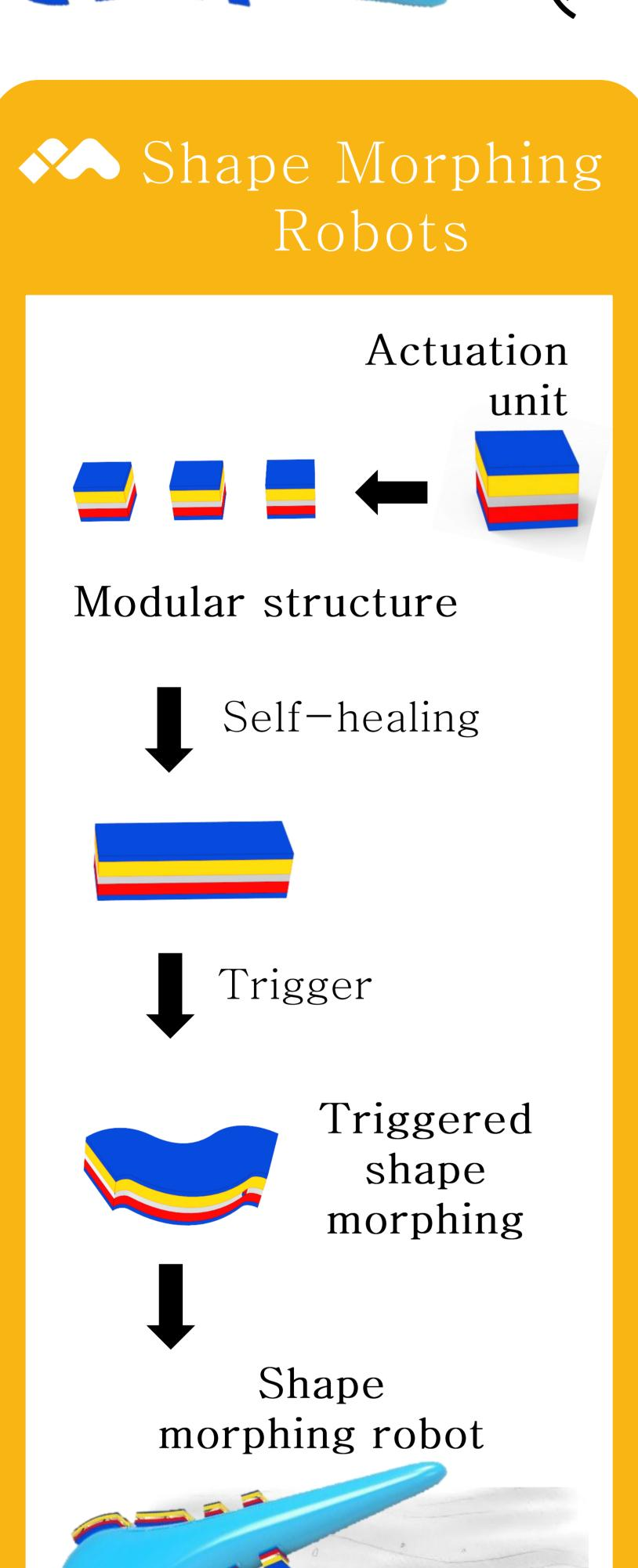
Developing modular robots able to change their shape. These modular robots will stand out for their self-adaptability to the environment and shape morphing capabilities.
