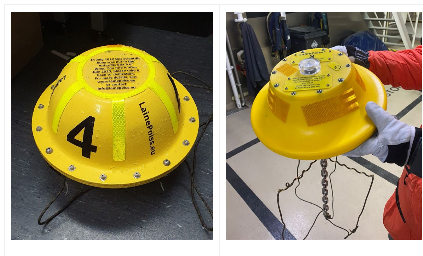
Figure 100 Three LainePoiss buoys were deployed as drifters during the SCALE WIN2022 cruise. (left) First generation of buoy made from fibreglass (LP2, LP4). (right) Second generation of buoy made from plastic (LP8). Photos by JVB.
