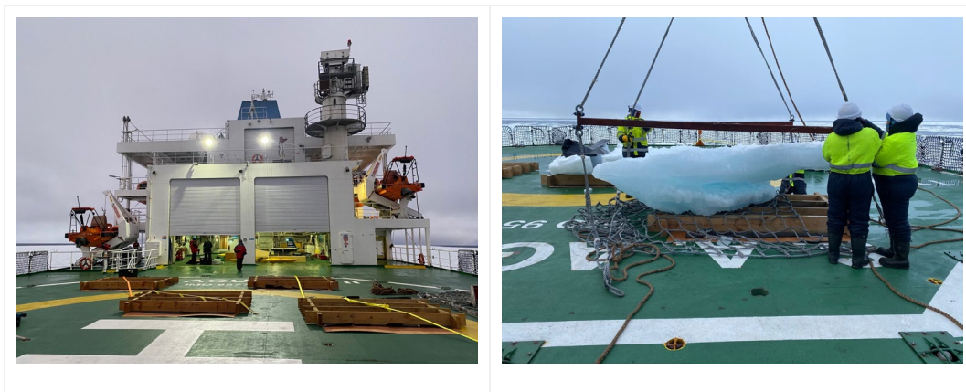
Figure 89 Pancake ice floe collection stations on the helideck on deck 5. (left) Four wooden lattices were constructed on the helideck and ice floes were placed on top of them for coring and imaging. (right) A pancake floe being lowered at OD-2. Photos by RV.
