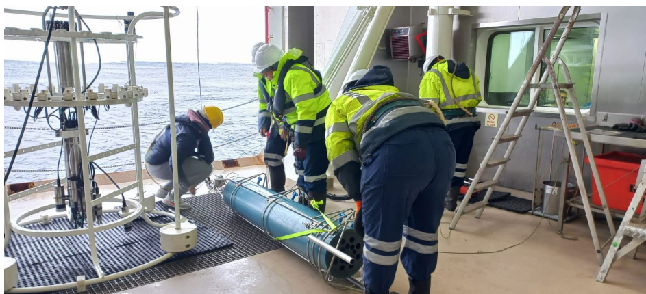
Figure 34 Prepping the Marine Snow Catcher for deployment. The messenger trigger mechanism requires careful handling. Photo credit: L. Lain
