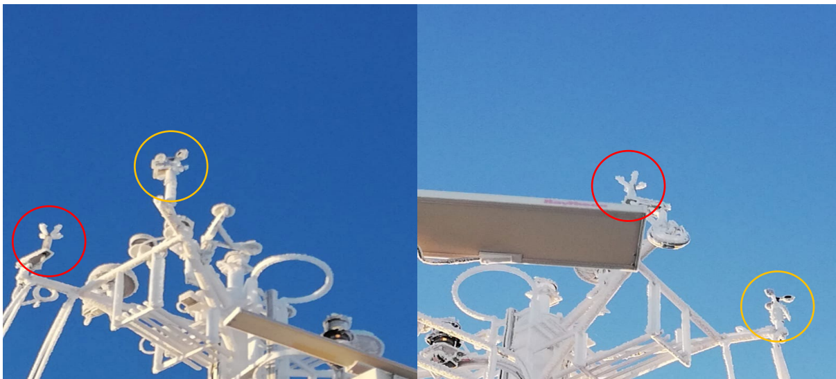
Figure 16. SAWS's ultrasonic wind sensor (circled in red) and the SDS mechanical wind sensor (circled in yellow) during the time at which they were frozen.
