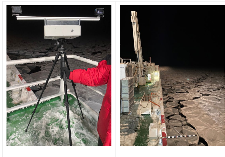
Figure 94 Stereo GoPro rig for imaging the UCT SHARC buoy deployment and retrievals.
