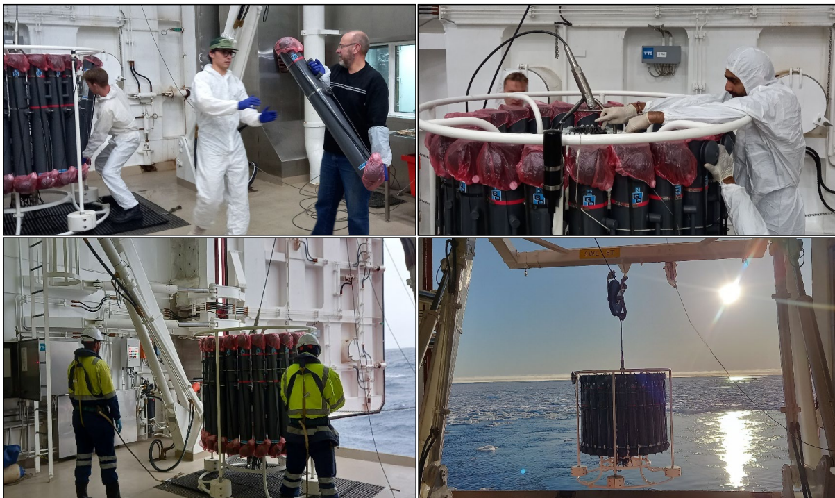
Figure 110. GoFlo deployment. Top: Transport of Go-Flo bottles to the rosette and preparing Go-Flo triggers before deployment; Bottom: Deployment in open water and marginal ice zone. Photo credit: S. Fietz
