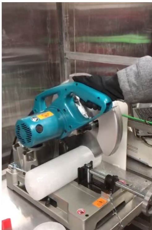
Figure 73 Makita M2401B 2000W cut-off saw in use
