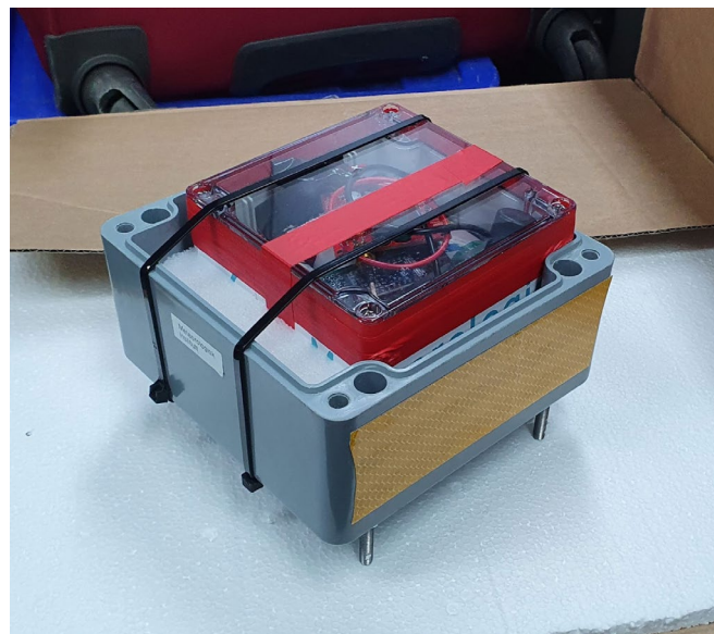
Figure 101 The FMI ice-tethered buoy (BB01) in its enclosure. The platform is based on the OpenMetBuoy-v2021 (Rabault et al. 2020) design. Photo by JVB.
