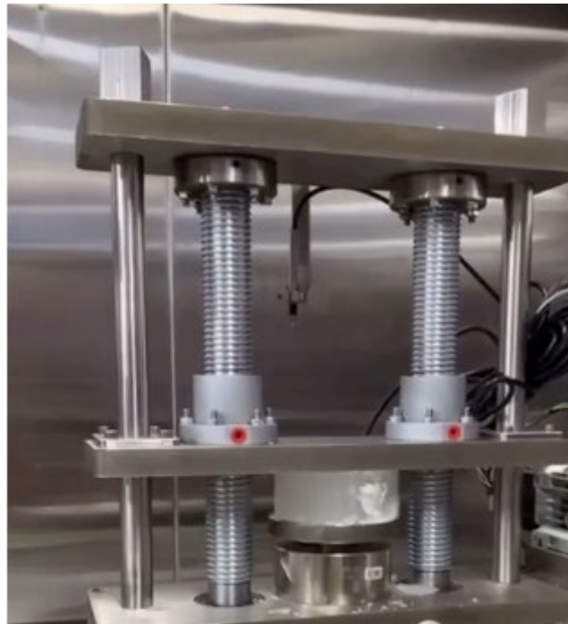
Figure 74 Electronically driven uniaxial compression device
