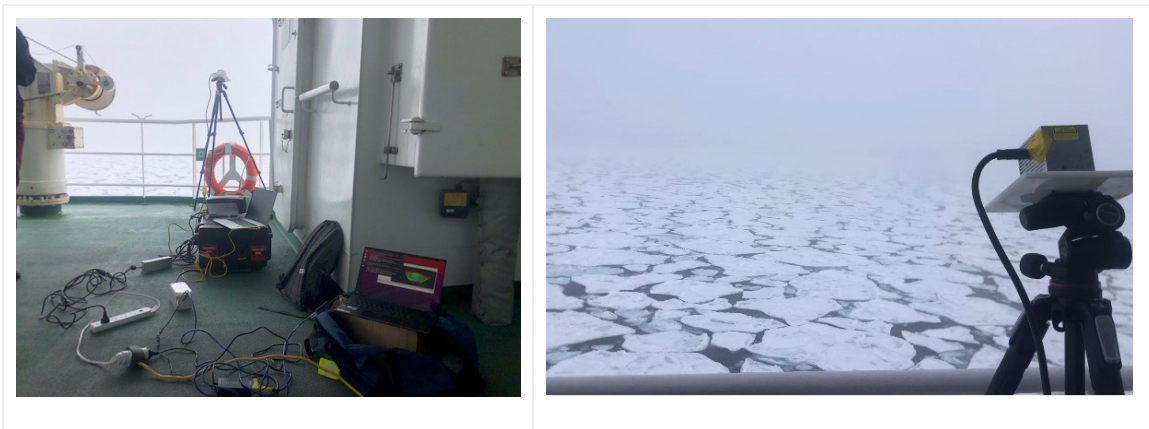
Figure 86 Full Livox Avia LiDAR setup installed on deck 7 for ocean and sea ice elevation monitoring. (left) installed on deck 7 alongside the thermal imaging rig; (right) the Livox Avia LiDAR attached to a tripod with a view of the sea ice field. Photos by AS.
