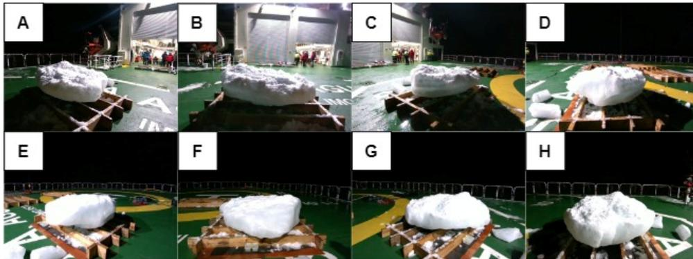
Figure 91 Scan positions around a pancake floe placed on the wooden lattice on the helideck. LiDAR and Realsense acquisitions were taken at each position and the distance from the floe was recorded.
