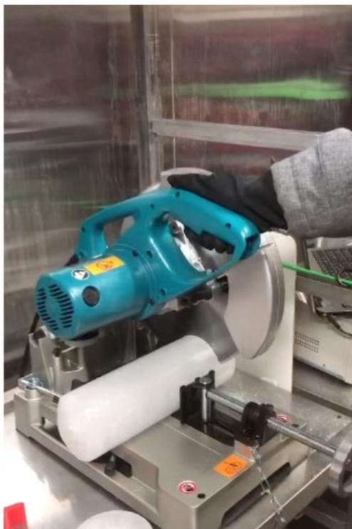
Figure 73 Makita M2401B 2000W cut-off saw in use
