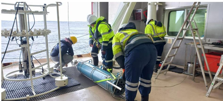
Figure 34 Prepping the Marine Snow Catcher for deployment. The messenger trigger mechanism requires careful handling.
