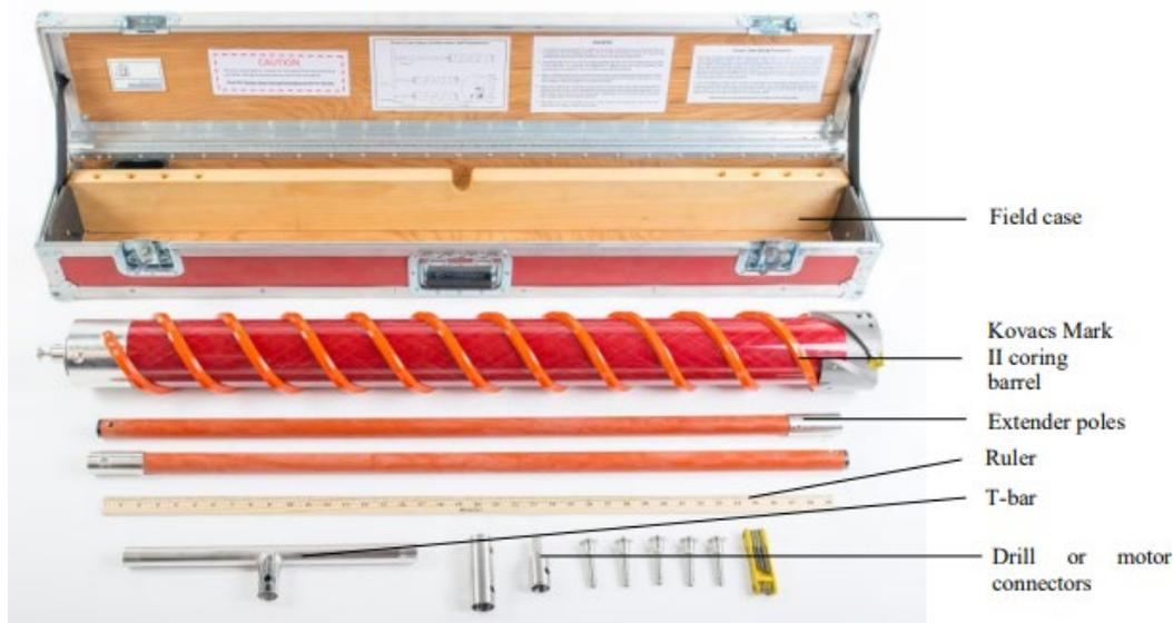
Figure 72 Kovacs Mark II Corer apparatus
