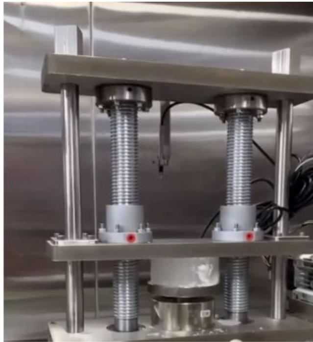
*Figure 74 Electronically driven uniaxial compression device*
