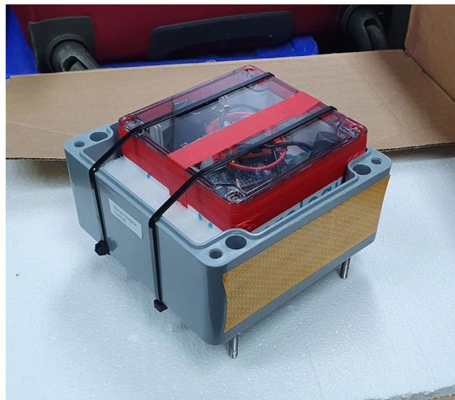
Figure 101 The FMI ice-tethered buoy (BB01) in its enclosure. The platform is based on the OpenMetBuoy-v2021 (Rabault et al. 2020) design. Photo by JVB.
