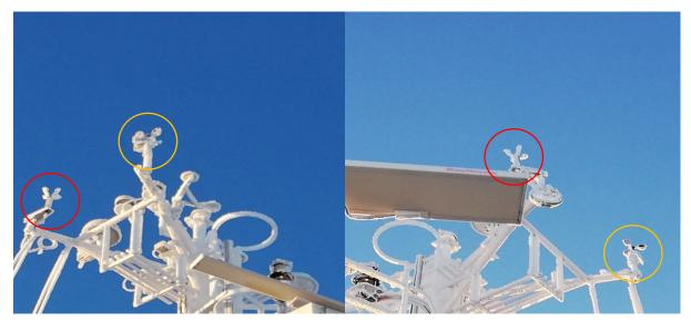
Figure 16. SAWS's ultrasonic wind sensor (circled in red) and the SDS mechanical wind sensor (circled in yellow) during the time at which they were frozen.
