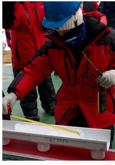
Figure 76 temperature measurements on deck after the collection of a pancake ice core
