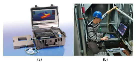
Figure 47: (a) Qass Optimizer4D; (b) AE System Installed at Shaft Line of the SA Agulhas II.
