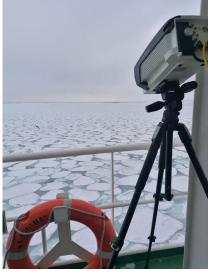
Figure 79 Setup for open ocean and sea ice surface temperature measurements from deck 7.
