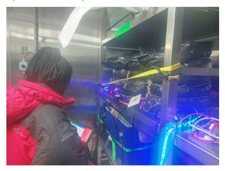
Figure 77 Algae Incubation Tank Set-Up in Processing Laboratory Freezer
