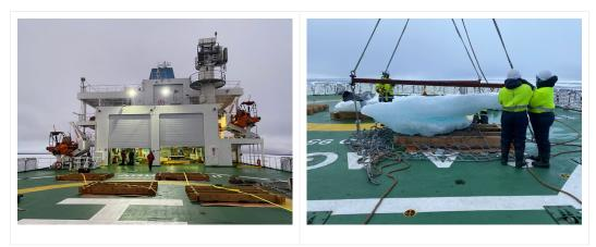
Figure 89 Pancake ice floe collection stations on the helideck on deck 5. (left) Four wooden lattices were constructed on the helideck and ice floes were placed on top of them for coring and imaging. (right) A pancake floe being lowered at OD-2.
