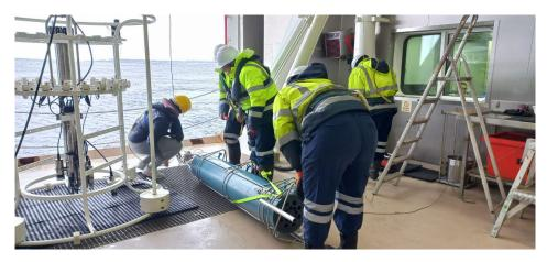
Figure 34 Prepping the Marine Snow Catcher for deployment. The messenger trigger mechanism requires careful handling.
