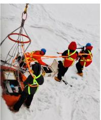
Figure 39 Spectral radiometer (TriOS RAMSES) with the custom-made beam and testing in the field
