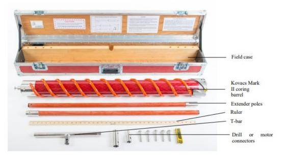
Figure 72 Kovacs Mark II Corer apparatus
