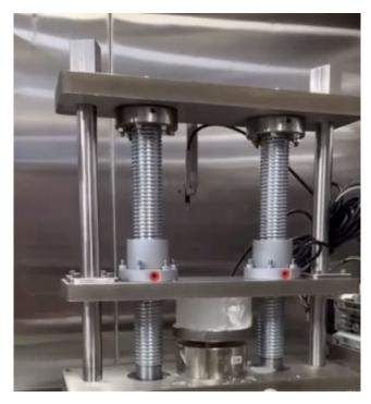
Figure 74 Electronically driven uniaxial compression device
