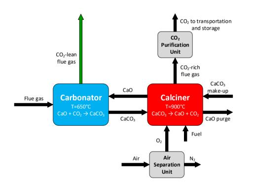
The flue gas stream produced by a real oxyfuel combustion is not a CO<sub>2</sub> – H<sub>2</sub>O binary mixture (because of air leakages, ASU efficiency, actual fuel and sorbent composition...)
