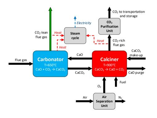
Given the high temperatures involved in the process, heat can be efficiently recovered in a steam cycle to produce electricity, thus decreasing the electricity consumption of the capture process
