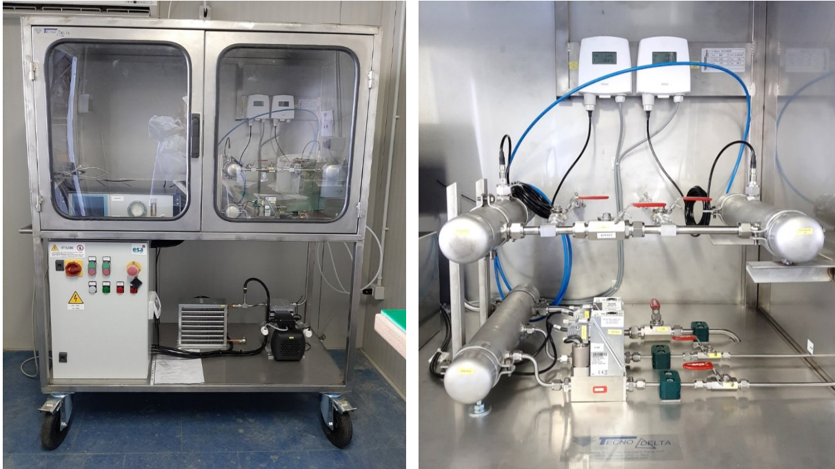
Figure 3: Testing equipment (flowmeters, mixing chambers, RH/T probes, by-pass connections, CO 2 analyzer) shown from the side (left) and from the top (right) (Usta et al, 2021).
