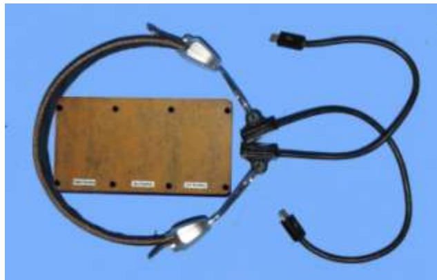
Figure 2:- Accelerometer attached to a headphone band.
