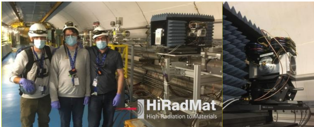
Figure 5: The waveguide EO-BPM installed in the HiRadMat (TNC) facility at CERN for beam tests with single-shot bunch trains.
