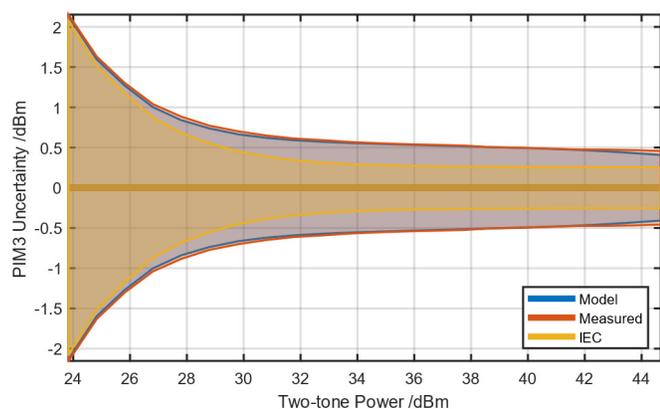
Fig. 7. PIM3 uncertainty calculated using the proposed methods and the IEC 62037-1 method.
