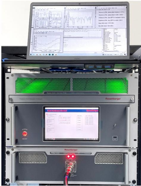
Fig. 1. Vector PIM measurement system in use at PTB.
