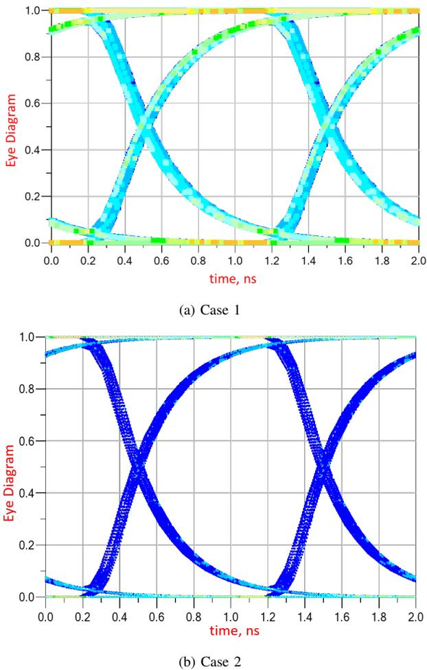
Fig. 6. Eye diagrams obtained for the considered digital signaling system working at 1 Gbps, in the mismatched case.
