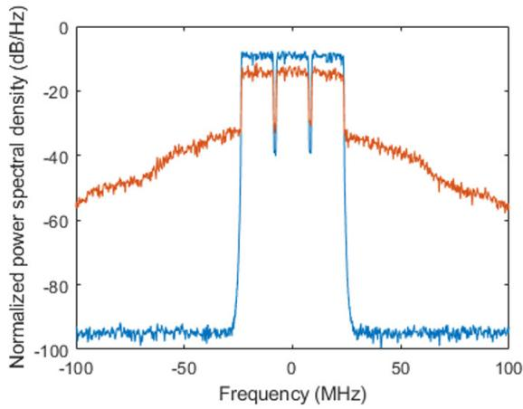
Fig. 4. Frequency spectrum of input signal (blue) and resulting output signal (red) under the load condition of Fig. 3.
