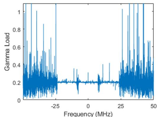
Fig. 3. Load reflection coefficient vs frequency after the emulation load pull algorithm has converged.
