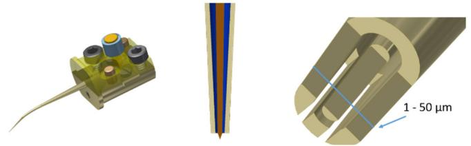
Fig. 2. Left: design of probe with holder. Center: probe construction, brown: PtIr inner conductor, blue: quartz glass dielectric, green beige: deposited Pt as outer conductor. Right: Ground-Signal-Ground structure at the probe's tip.
