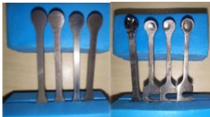
Fig. 20 Unused and used tantalum electrodes
