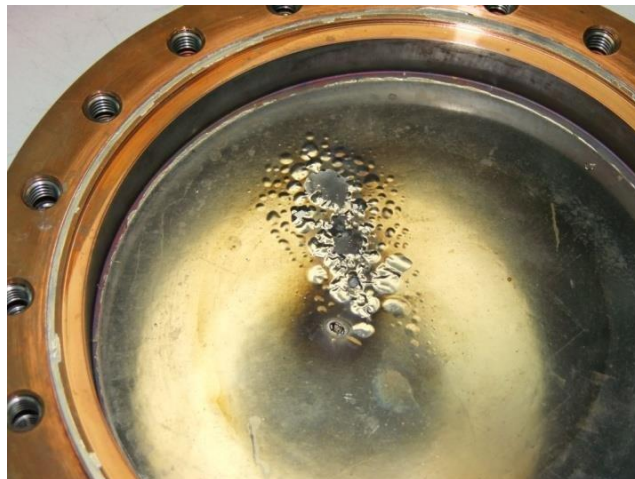
Fig. 7 A 40 cm diameter tungsten beam dump from SARAF accelerator damaged after several minutes of irradiation by 4 MeV protons at a current of 6 \times 10^{15} protons/sec [15]
