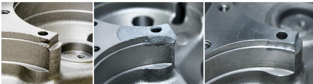
Fig. 15 Cold spray AM repair process of flange – damaged part, part after spraying, part after machining [36]
