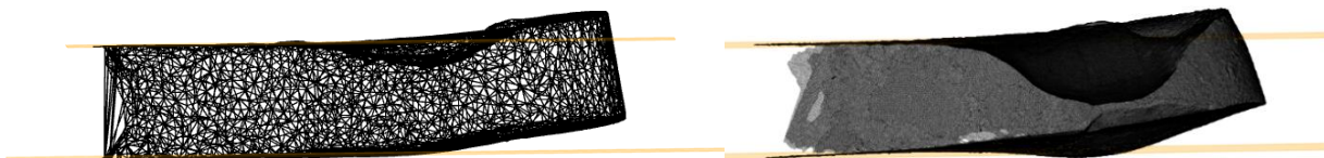
Fig. 23 Electrode shape deformation 3D scan
