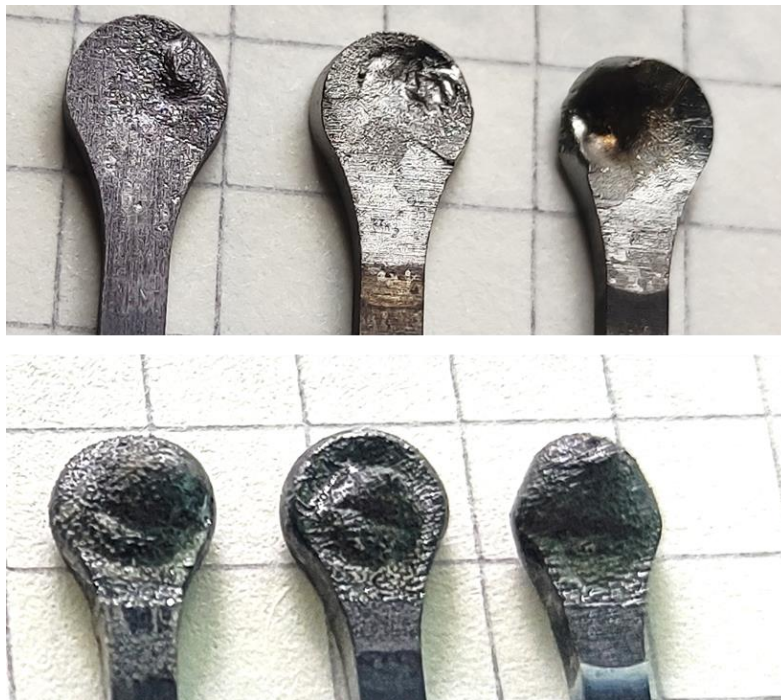
Fig. 29 Damaged electrodes (top) and repaired electrodes(bottom) using powder DED
