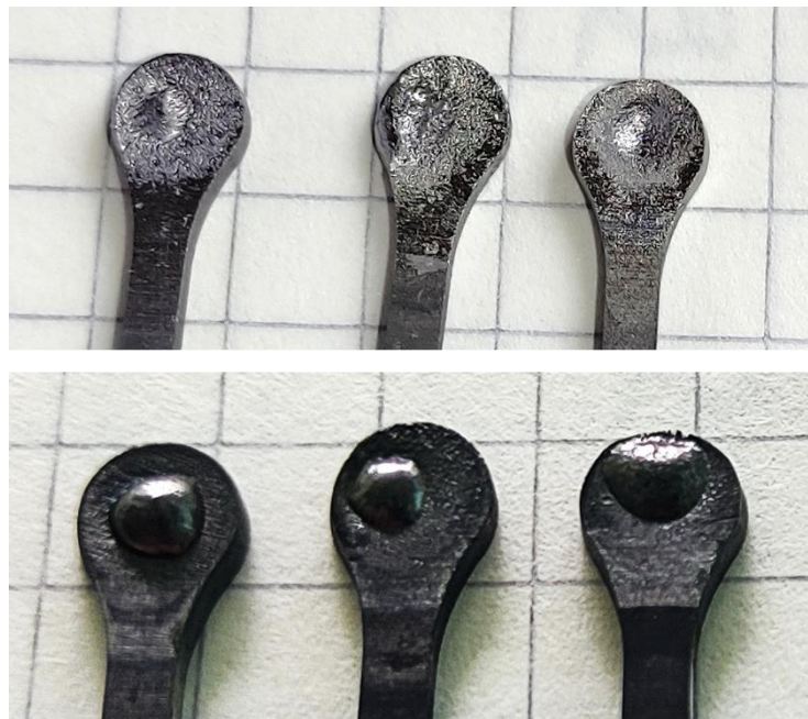
Fig. 28 Damaged electrodes (top) and repaired electrodes(bottom) using wire DED
