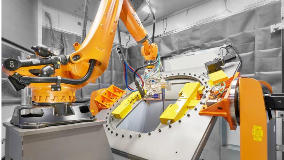
Fig. 19 AM setup with KUKA shelf-mounted robots [44]
