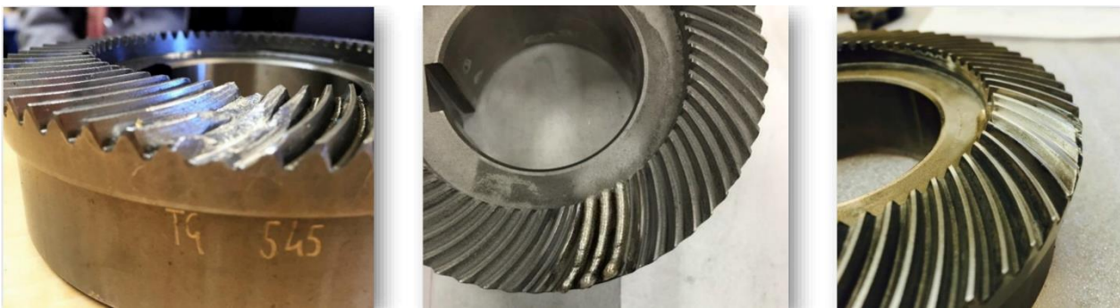
Fig. 1 Additive repair process of broken gear teeth: broken gear teeth, additive repair process and finished machined part (left to right) [2]
