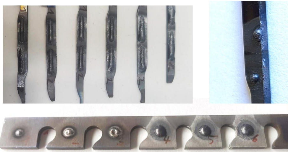
Fig. 26 Different test shapes manufactured by powder DED
