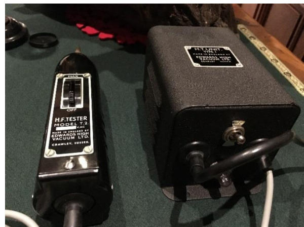
Figures 2.23 and 2.24. Portable Tesla Coil used in experiment for X-rays production from Tesla Tube with single
