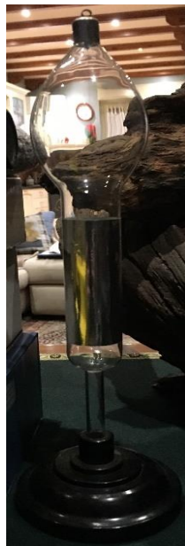
Figure 2.21. Single node Tesla Tube, from Industrie Italiane Galileo, used in experiment, with basal support and single node localized in upper part of tube, near of ampullary enlargement
