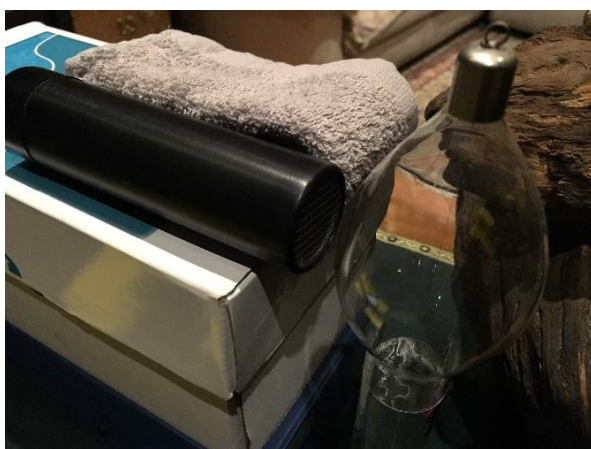
Figures 2.25 and 2.26. Detail of the proximity of the external probe of the Mueller Geiger Counter, to the ampullary enlargement of the Tesla tube, where it is assumed, thanks to the internal protusion of the cathode, that
