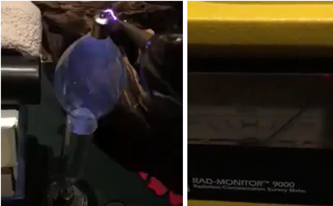
Figures 2.27 and 2.28. The image on the left shows the luminescence of the low pressure gas, inside the tube, excited by the high ddp discharge, provided by the Tesla Coil, where we see the spark exiting the secondary, at the upper apex of the tube, which activates the cathode. The image on the right, unfortunately grainy, shows the level of X radiation detected by the Geiger counter. The detector needle is over half of the reading index. (The image is grainy as it was taken from a still image of a video, shot by the author himself, during the execution of the experiments) - Courtesy of Stefano Turini's Private Collection
