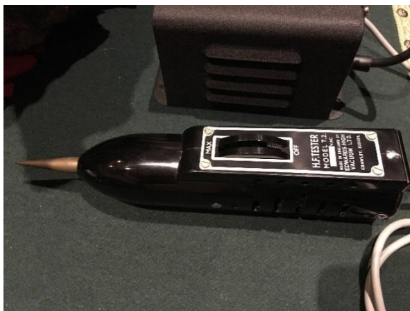
Figures 2.23 and 2.24. Portable Tesla Coil used in experiment for X-rays production from Tesla Tube with single
