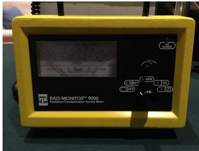
Figure 2.22. Geiger Counter detector, with external probe, used for detection of X-rays from Tesla Tube
