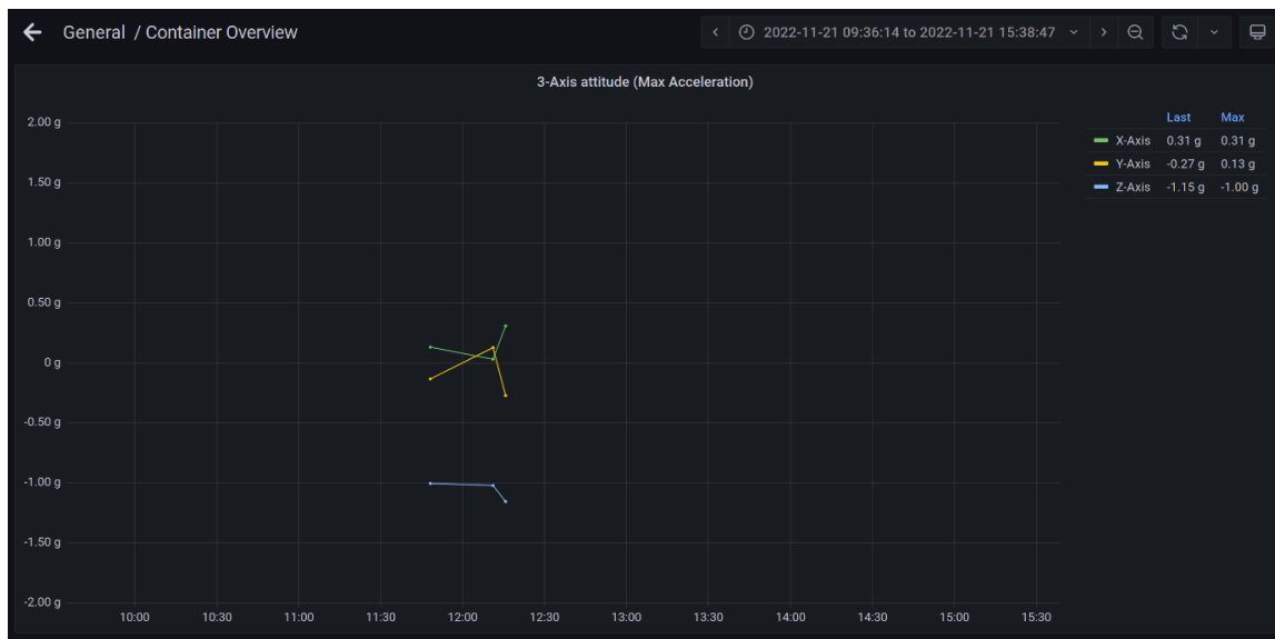
Figure 61: Accelerometer measured in real-time in the Port of Valencia on 21 November 2022
