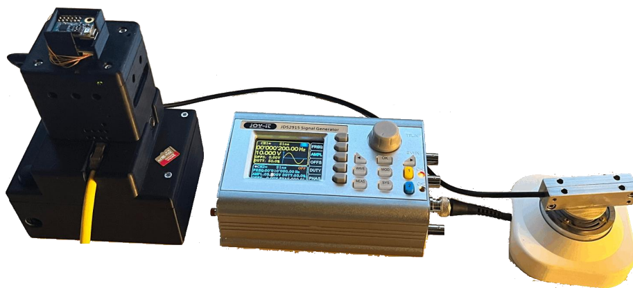
Figure 12: Rail-Health Simulated Fault & Sinusoidal Fault Injector Set-up
