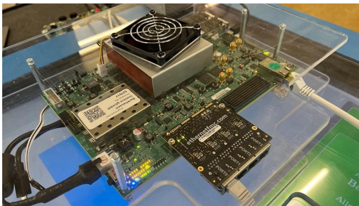
Figure 13: BI's M 3 hardware/software co-design platform realized on FPGA development board, with external Ethernet extension board
