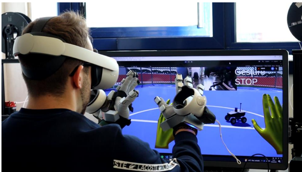
Figure 42: Remote cockpit including the SensGlove haptic gloves, VR glasses and Digital Twin.
