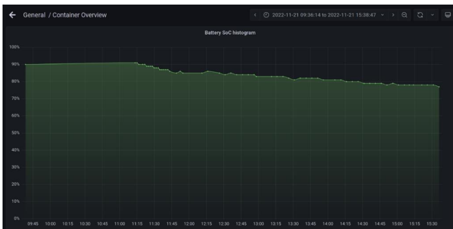
Figure 59: Battery state of charge of the IoT devices, measured in real-time in the Port of Valencia on 21 November 2022
