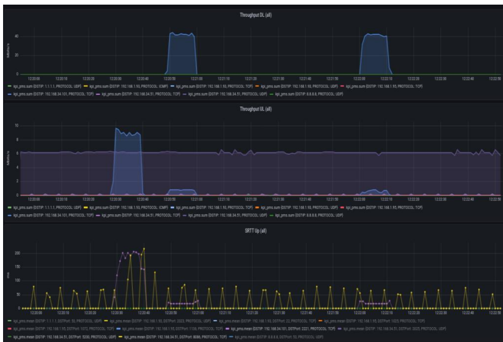
Figure 8: Grafana KPI dashboard visualization of UE to core with video streaming running. 1) Top: Downlink throughput – iperf3 test (Blue). 2) Middle: Uplink throughput – iperf3 test (Blue) and video streaming (Purple). 3) Bottom: RTT uplink – influxDB connection (Yellow) and iperf3 test (Purple).
