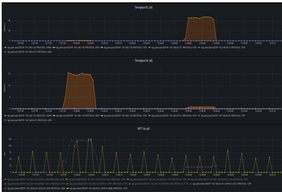
Figure 7: Grafana KPI dashboard visualization of UE to core without video streaming running. 1) Top: Downlink throughput – iperf3 test (Orange). 2) Middle: Uplink throughput – iperf3 test (Orange). 3) Bottom: RTT uplink – influxDB connection (Yellow) and iperf3 test (Purple).
