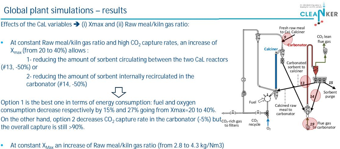
determines an increase of the overall carbon capture rate (>95%) but involves also an increase of fuel and  $O_2$  consumption (respectively +26% and +30%), required for calcining a higher amount of fresh sorbent.
