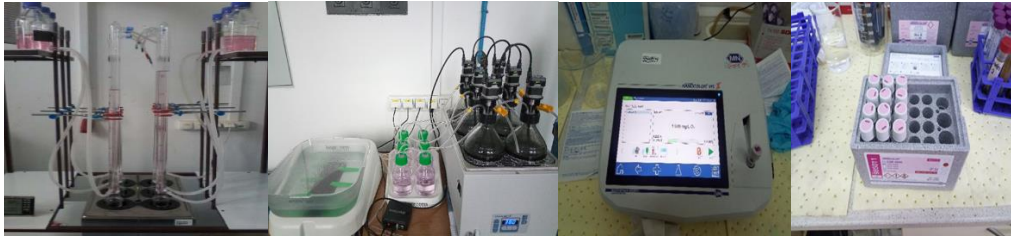
Fig.4 DIN 38414/8 eudiometers used for small-scale (400 ml) experiments including water bath, A view of the AMPTS II device used in the experiments. A photo of the analytical set used for the SCOD measurements: Macherey–Nagel photometer, photometric tests—tubes filled with appropriate reagents (from left to the right).
