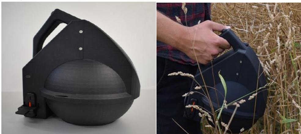
Figure 42. VideometerLite, portable handheld multispectral imaging device.
