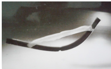
○ Fig. 3.21 Shrinkage of the polymer after drying
