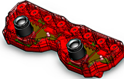
○ Fig. 5.18 Stereoscopic kit with two digital cameras
