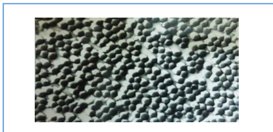
Fig. 3.31 Surface of ultrathin film of BM-12 acrylate suspension (x13000, electron microscopy)
