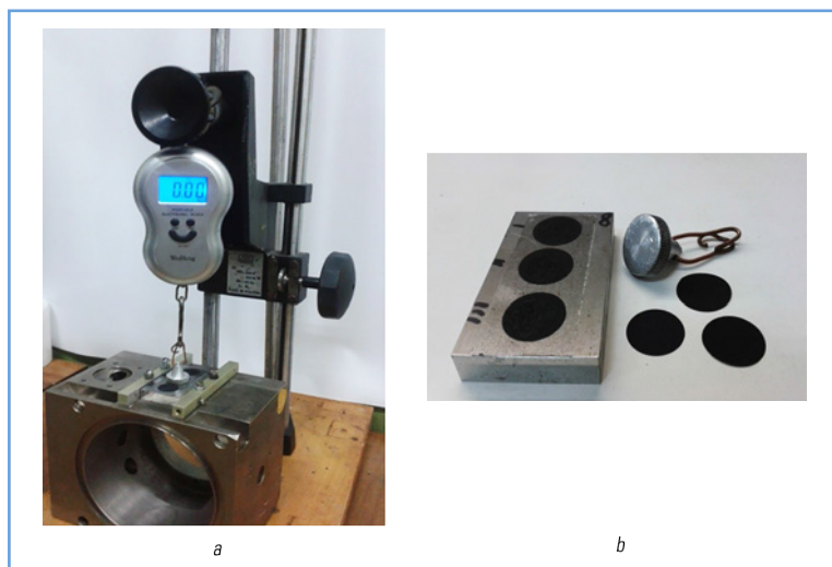
Fig. 3.8 Laboratory unit for measuring the amount of force applied to detach the sample from the surface of the base: a – a device for measuring the adhesion of a composite material to a substrate; b – a steel plate with glued samples and a metal nickel of the same diameter, for peeling off with a load
