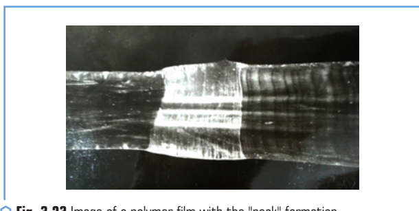
Fig. 3.23 Image of a polymer film with the "neck" formation
