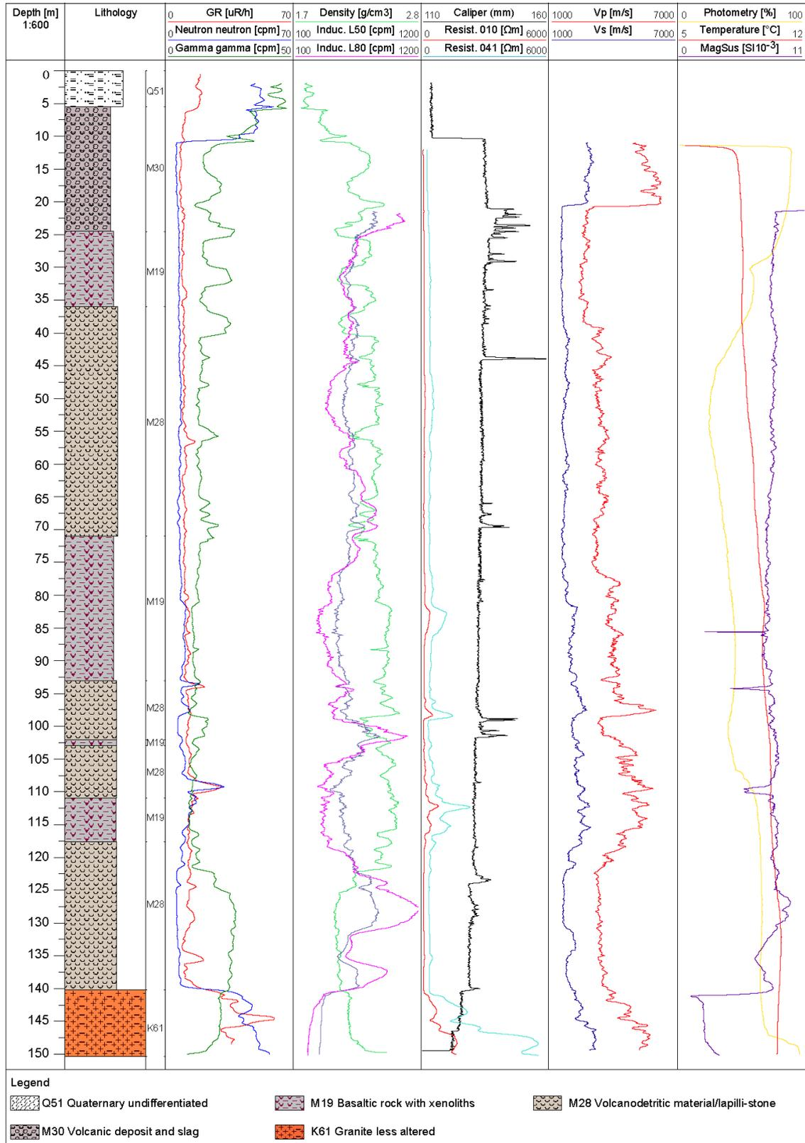
The stratigraphy profile and logging data of the S4b borehole. GR stands for natural gamma ray.
