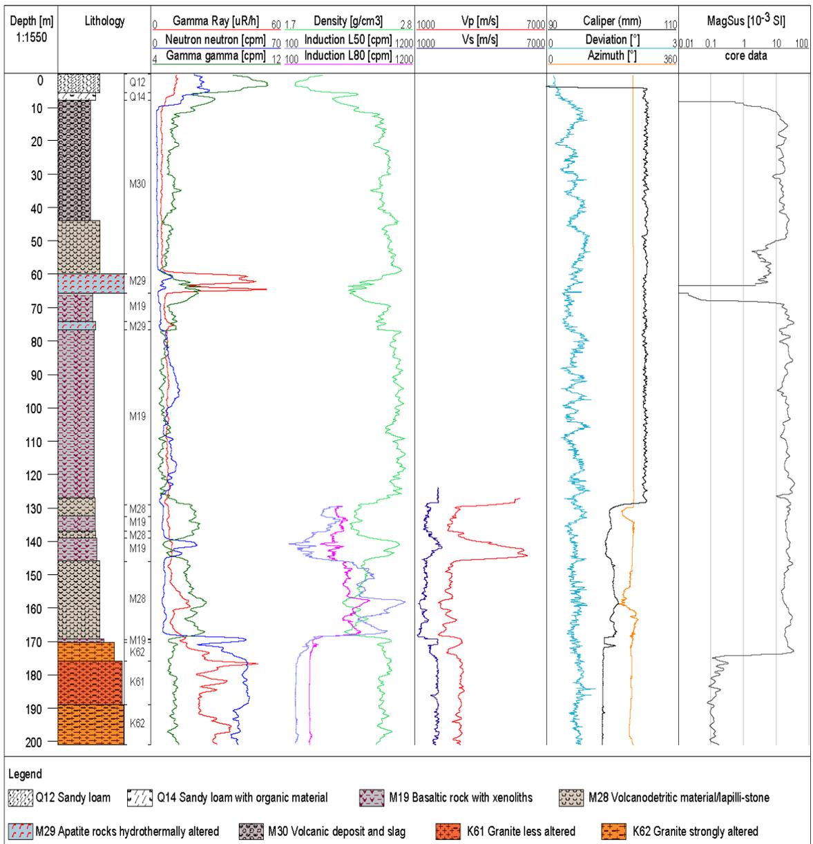
The stratigraphy profile and logging data of the S4 borehole in the depth range of 0–200 m. The Vp, Vs and Inductions data in a depth range of 0–130 m were not acquired due to the presence of provisional casing supporting the borehole.
