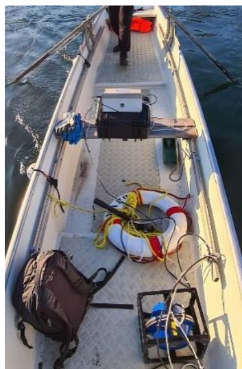
Figure 10. Installation of the acoustic source on a rowboat. The blue device on the bottom is the underwater speaker. The black box on the bench contains the electronics and batteries. On top of the box is a tablet computer to control the broadcasts.
