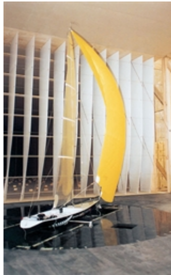
Figure 2.10: Picture of the Twisted Flow Wind Tunnel (TFWT), at the University of Auckland SW, in New Zealand, which is an open circuit wind tunnel; equipped with vertical turning vanes that can be twisted and generate twisted flow. The picture is published with the approval of Professor Richard GJ Flay, at The University of Auckland, New Zealand.
