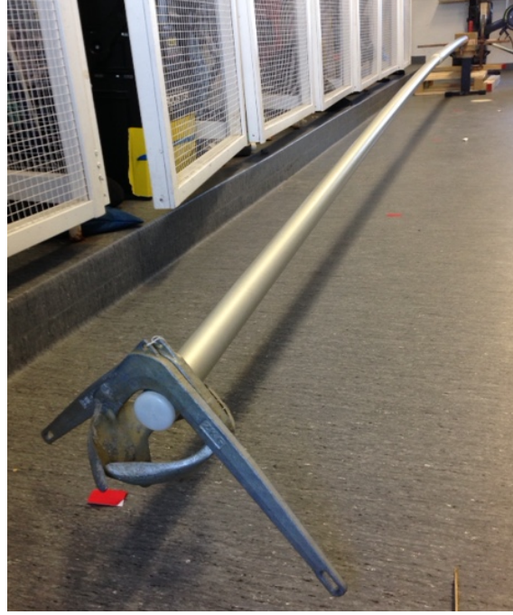
Figure 4.4: Flexural tests of the ILCA 7 mast, for the analysis of the displacement curve.
