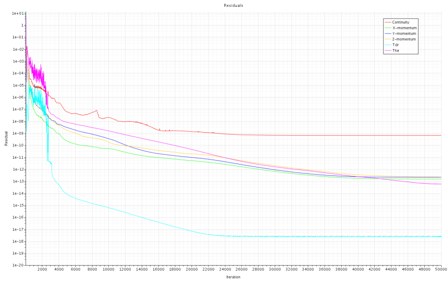
Figure A.105: Residual vs iteration, from the RANS simulations performed with the flat sail model, with a sheet angle of 90^\circ , in the large computational domain & grid 1, showing the graphs of the Continuity (red), X-momentum (green), Y-momentum (blue), Z-momentum (yellow), Turbulent dissipation rate (cyan) and the Turbulent kinetic energy (purple).
