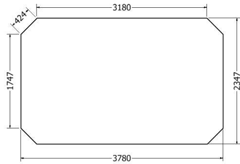
Figure 4.22: Cross sectional dimensions [mm] of the inlet, of the large computational domain.
