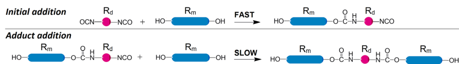
Scheme 3 Two stages of the polyaddition of diisocyanates to the excess macrodiols. Top: initial addition as the very first reaction to form a monofunctional adduct of large molecular size. Bottom: adduct addition as the second reaction, which prevails due to macrodiol excess. Further polyaddition is not shown.
