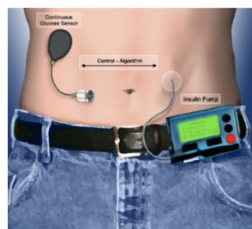
The Artificial Pancreas is actually a combination of internal glucose monitor, insulin pump, and control software.
