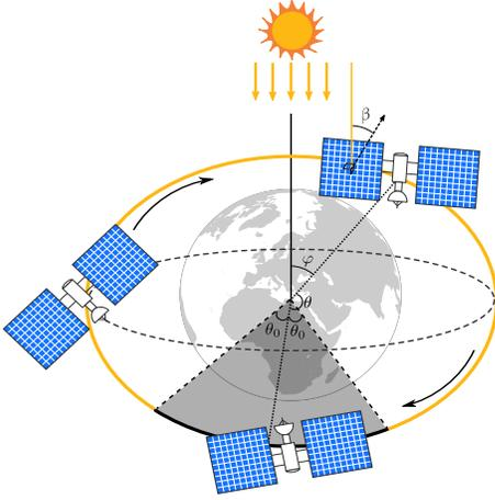
Fig. 1. Illustration of the LEO satellite's orbit.
