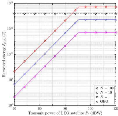
Fig. 4. Harvested energy by the gRA vs. the transmit power of LEO satellites.
