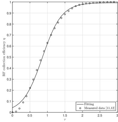
Fig. 3. RF collection efficiency as function of  $\tau$ .
