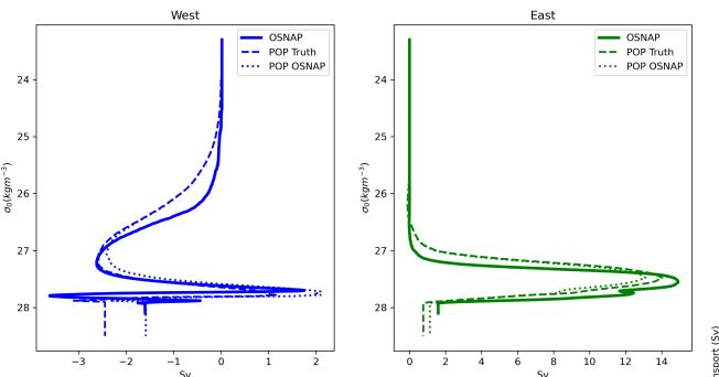
Model realistically captures the relative strengths of overturning in the east and west Preliminary results show good agreement between the model truth and the model observational equivalent
