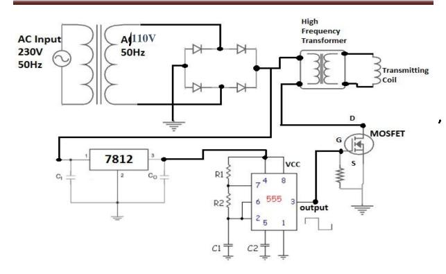
In above figure, Timer IC 555 is used to generate very high frequency of 864MHz and other parameters use as follows are:
