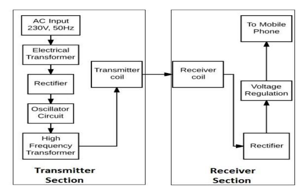
The receiver circuit receives the induced voltage within the receive
