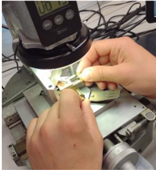
Figure 6: XY table adjustment
