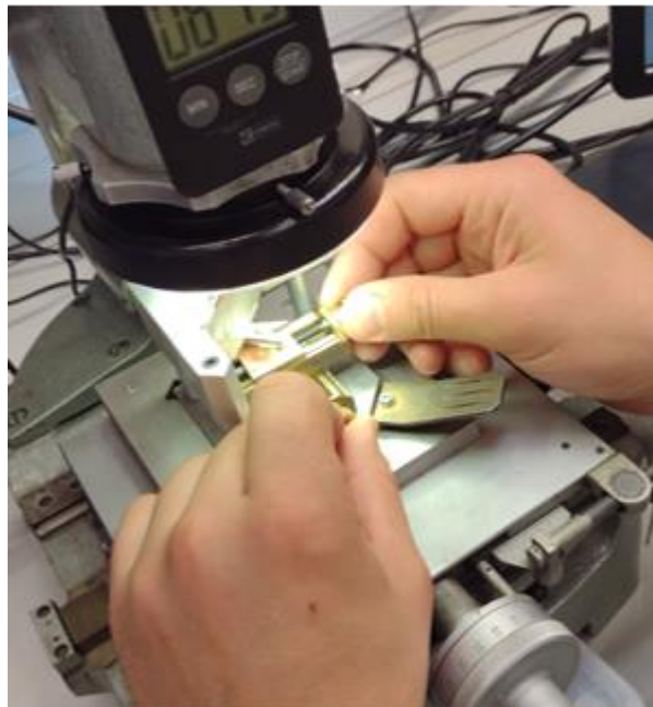
Figure 9: XY table movement to chip position
