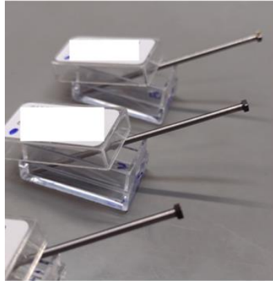
Figure 12: Chip glued to wire before machining
