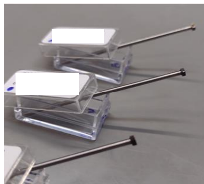
Figure 11: Chip glued to wire before machining
