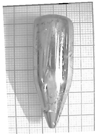
Fig. 4. As grown ingot of Ga<sub>0.9</sub>In<sub>0.1</sub>Sb
