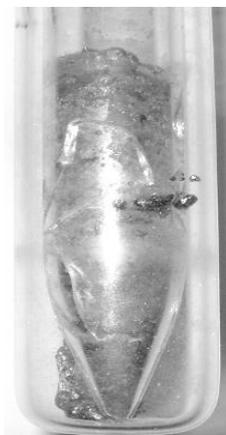
Fig.3. cracked ampoule wall
