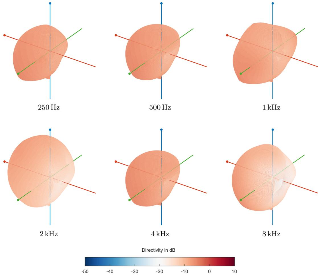
Figure 5: Balloon plots viewed from slightly backward and slightly upward ( $\phi = 215^\circ$ ,  $\theta = 30^\circ$ ) for the measurements from Dunn and Farnsworth [11]. Frequencies of 250 Hz, 500 Hz, 1 kHz, 2 kHz, 4 kHz, and 8 kHz are shown.
