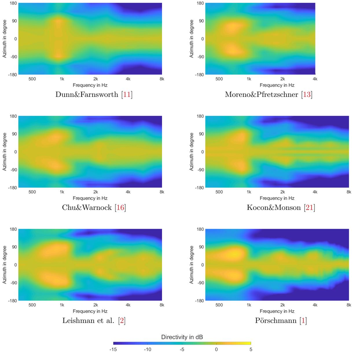
Figure 3: Directivity patterns over frequency in the horizontal plane for the measurements for which directivity patterns of fluent speech have been determined up to 8 kHz ([13] only up to 4 kHz).
