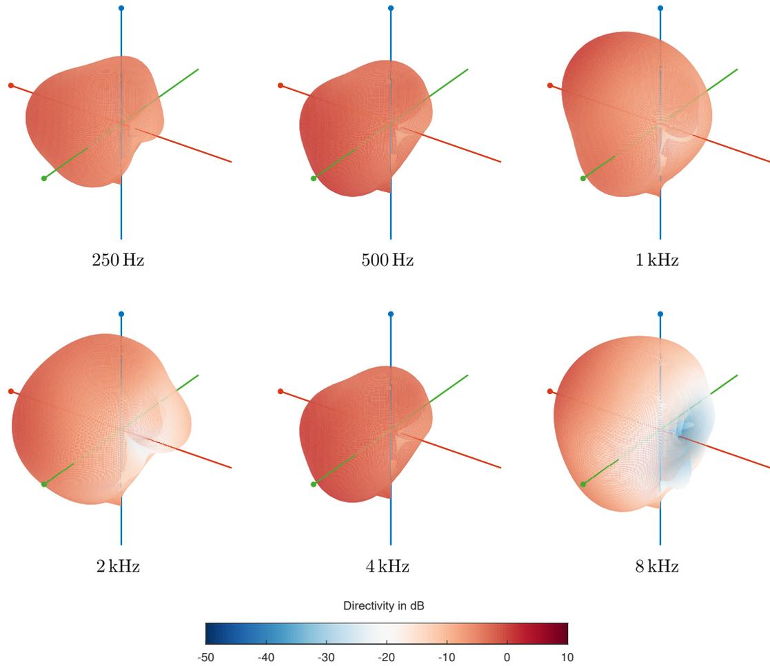
Figure 8: Balloon plots viewed from slightly backward and slightly upward ( $\phi = 215^\circ$ ,  $\theta = 30^\circ$ ) for the measurements from Pörschmann [1]. Frequencies of 250 Hz, 500 Hz, 1 kHz, 2 kHz, 4 kHz, and 8 kHz are shown.
