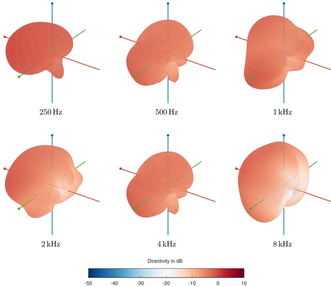
Figure 7: Balloon plots viewed from slightly backward and slightly upward ( $\phi = 215^\circ$ ,  $\theta = 30^\circ$ ) for the measurements from Leishman et al. [2]. Frequencies of 250 Hz, 500 Hz, 1 kHz, 2 kHz, 4 kHz, and 8 kHz are shown.
