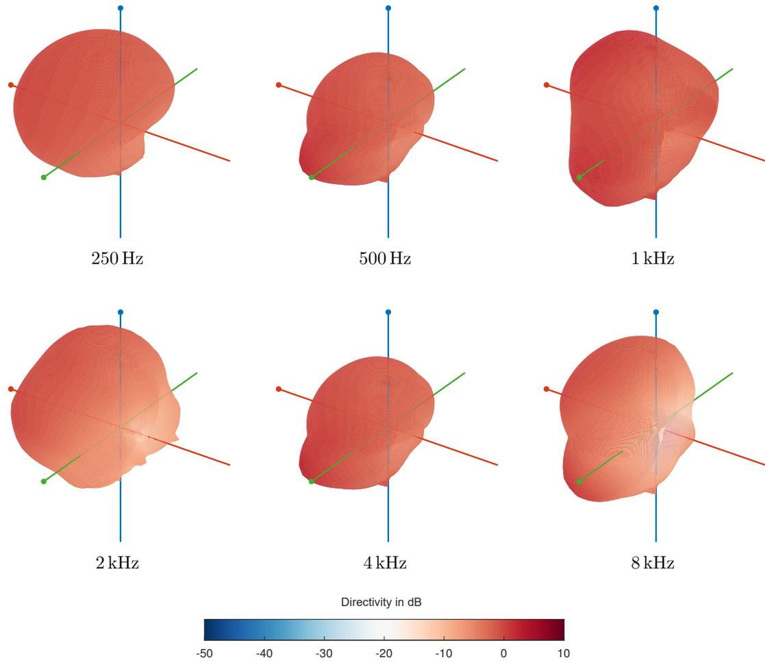
Figure 6: Balloon plots viewed from slightly backward and slightly upward ( $\phi = 215^\circ$ ,  $\theta = 30^\circ$ ) for the measurements from Chu and Warnock [16]. Frequencies of 250 Hz, 500 Hz, 1 kHz, 2 kHz, 4 kHz, and 8 kHz are shown.
