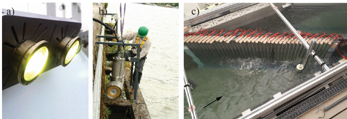
Figure 4.17 Variation of Sensory and behavioural measures on the field and in lab conditions. It presents LED lights for repelling fish at intakes (a), an Infrasound "canon" for repelling fish (b), and an Electrified Curved-Bar Rack – Bypass System (c) (Source: [4.31])
