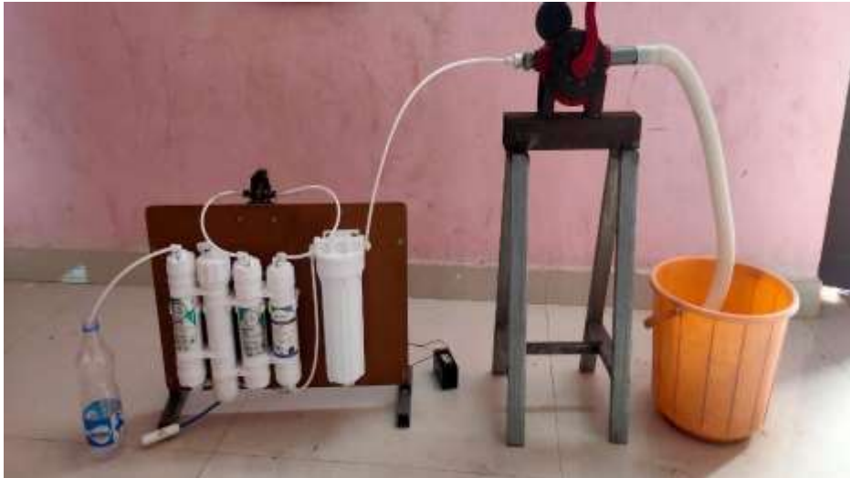
Fig. 1: Final assembly of pedal powered system.
