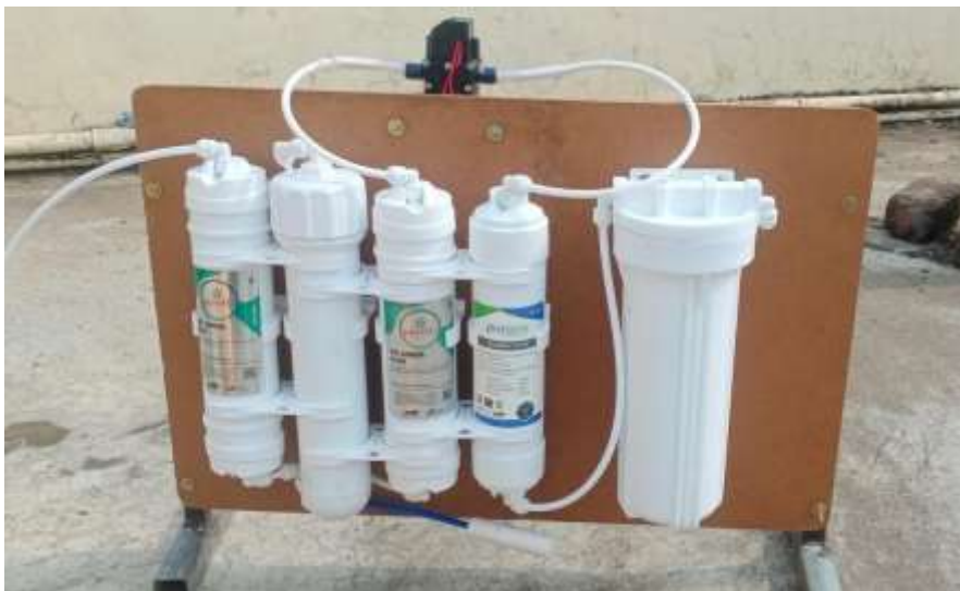
Fig. 2: Water filtration unit along with frame.
