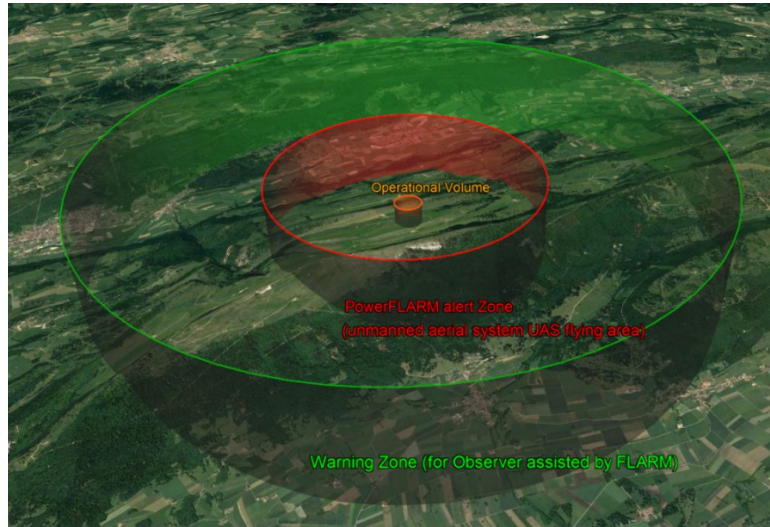
Figure 7: Alert zone parameters and visualization of the FLARM warning zones
