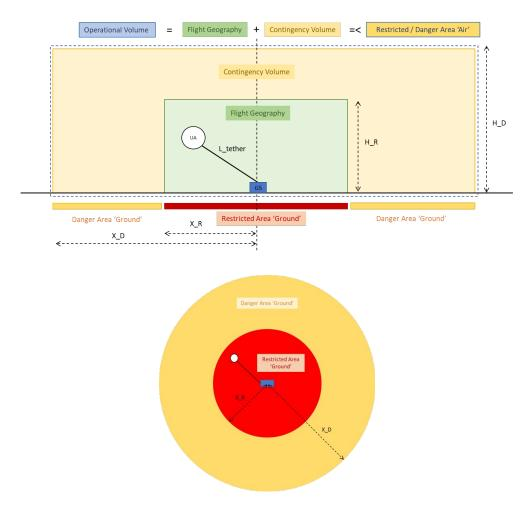
Figure 1: Definition and terminology to describe the AWE 'operational volume' (side and top view)
