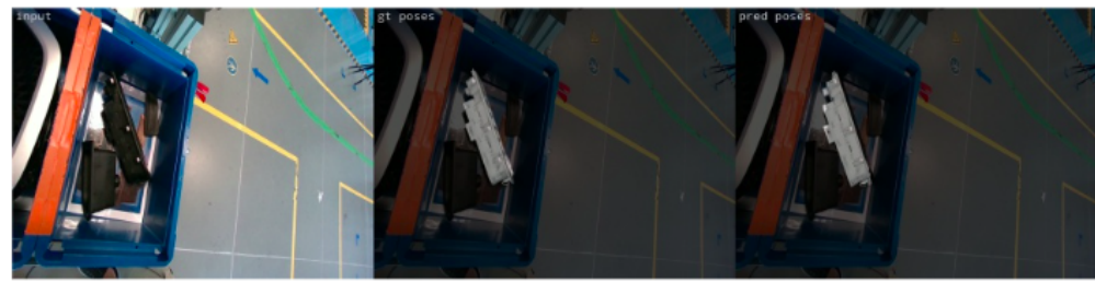
Figure 18. Examples of precise predictions on validation images from the real industrial environment. The first column presents the input validation image, the second column the ground truth, and the third one the estimated object pose.
