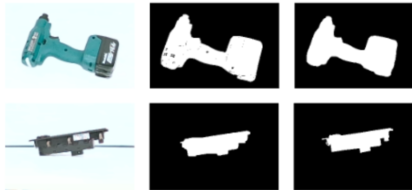
Figure 9. Closeups of examples of masks calculated by the standard EPOS masking method [45] (middle column) and U-Net (right column) along with the original image (left column).
