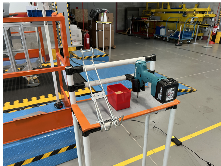
Figure 1. View of the assembly line depicting the screwdriver placement.
