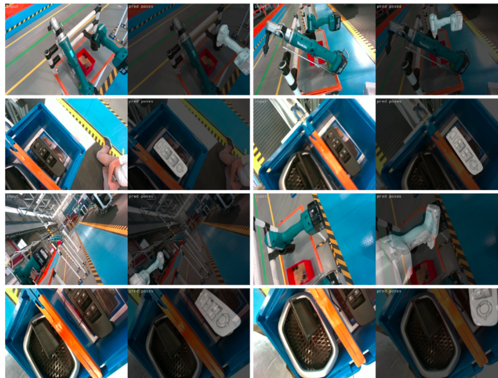
Figure 20. Examples of predictions on real test images. The first rows present correct object pose predictions, while the last two show incorrect ones.
