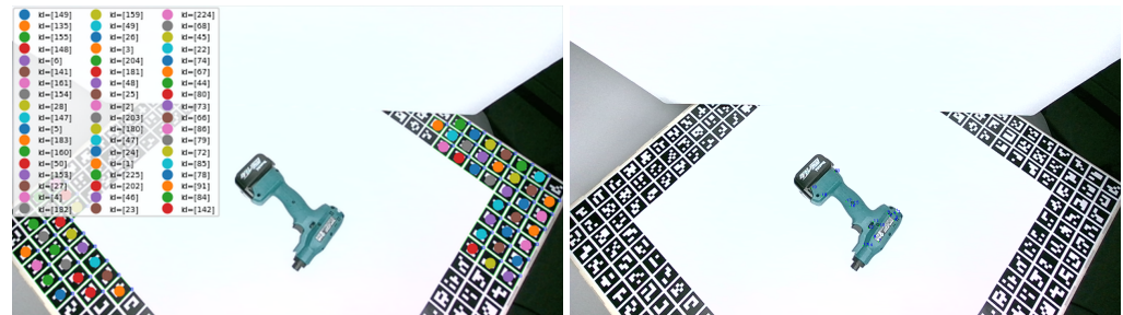
Figure 11. Automatically detected Aruco markers (left) and manually selected object points (right) on the training images, used to calculate the ground truth object pose.
