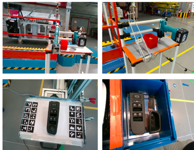
Figure 16. Sample training images from the real industrial environment dataset for the screwdriver (top row) and the window control panel (bottom row).
