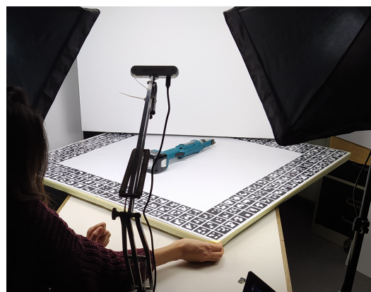
Figure 7. Setup prepared for capturing training and validation images in the laboratory. Objects are placed on a turnable table and the camera is mounted on an adjustable arm.
