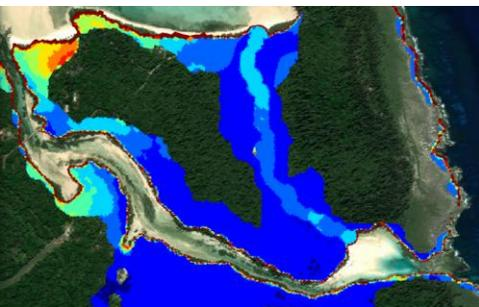
Tsunami runup: simulated current (m/s)
